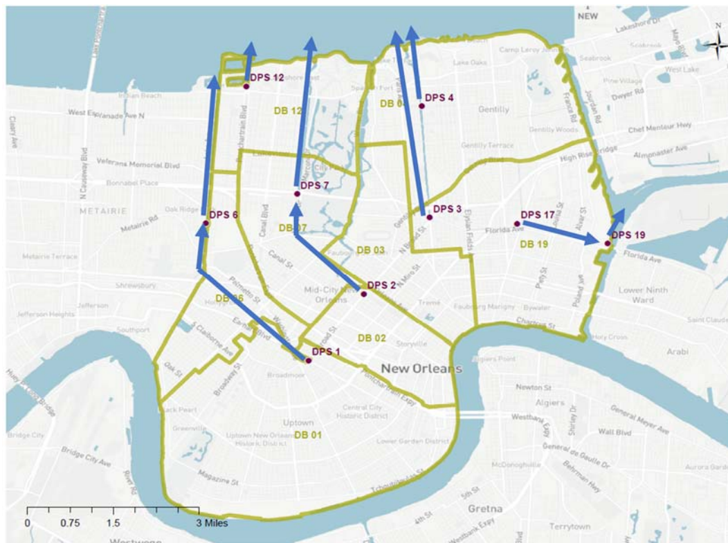
Figure 11 Drainage Pumping Stations and Discharge Paths
